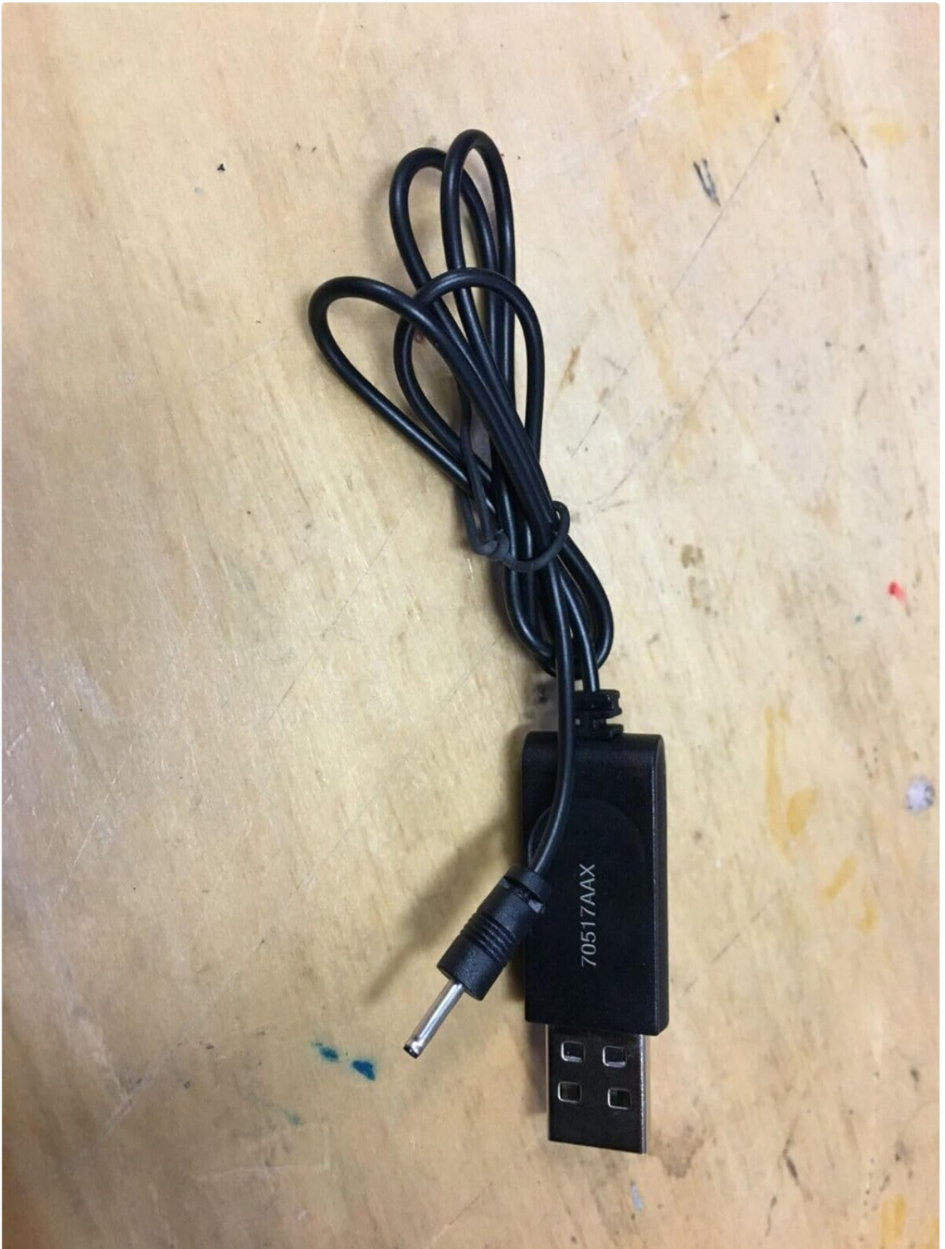
Image 1: Front view of the Generic USB Charger, showing the USB-A plug, cable, and barrel connector. The cable has a label "70517AAX".
