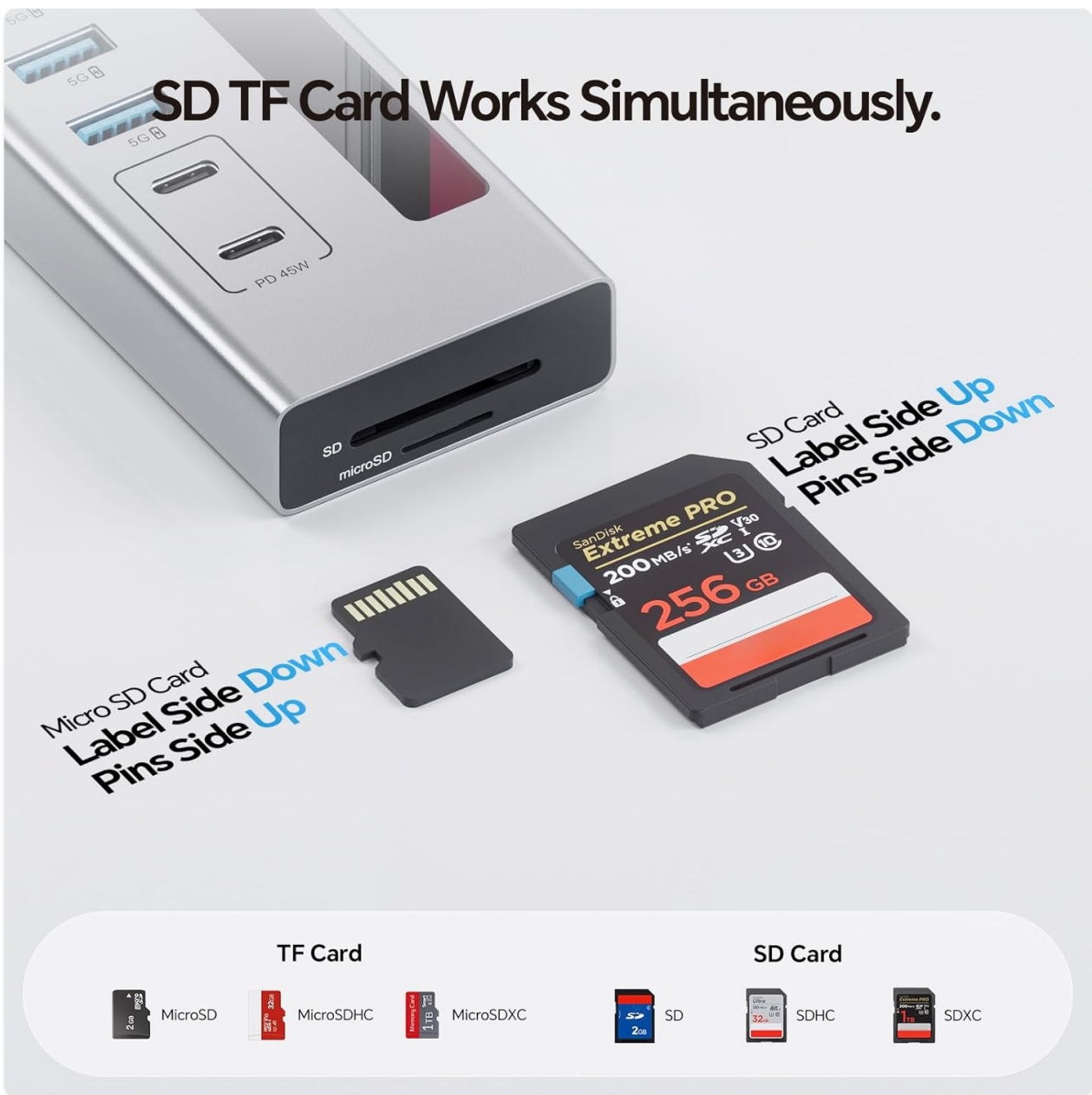
Image: Close-up of the SD and MicroSD card slots on the hub, illustrating simultaneous card usage.
