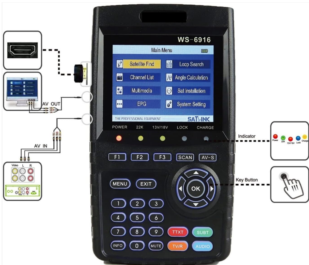
Figure 5: Connection diagram illustrating the AV IN and AV OUT ports, and how to connect them to external video and audio devices.
