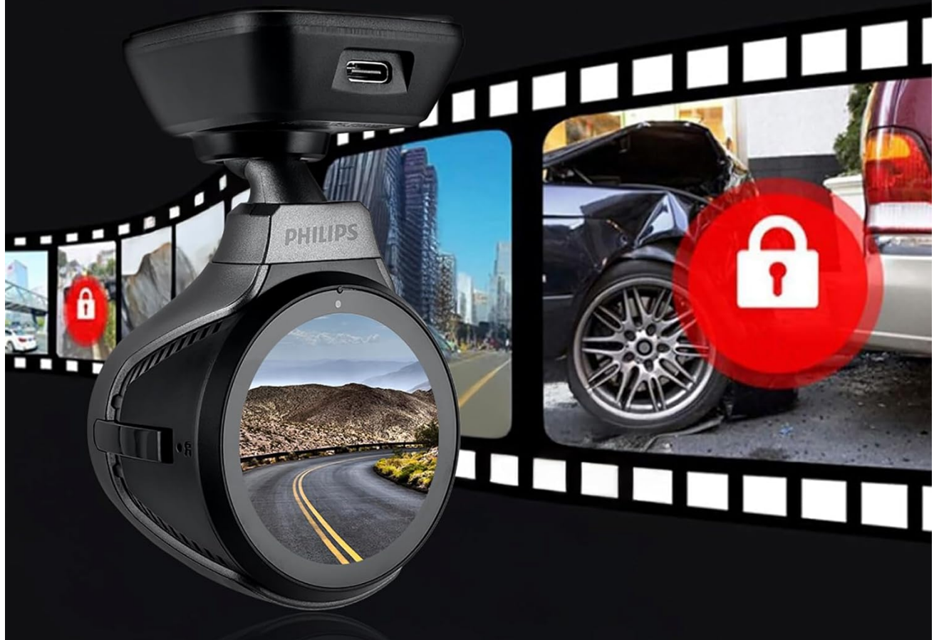
Image 4.2: Automatic Cycle (Loop Recording). This image illustrates the loop recording function, where the dash camera continuously records and automatically overwrites older files when storage is full. It also shows a locked file icon, indicating that G-sensor activated recordings are protected from being overwritten.
