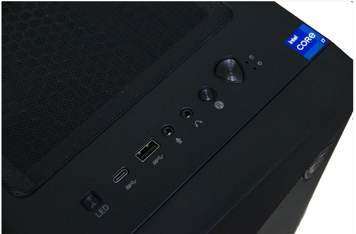
Figure 2: Top front panel of the desktop, showing the power button, USB ports, and audio jacks.
