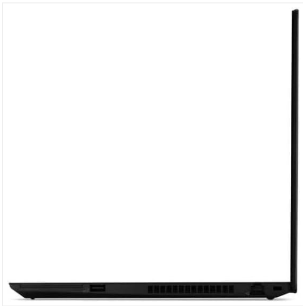
Figure 4: Right side profile of the laptop, showing the additional USB-A port and MicroSD card reader.
