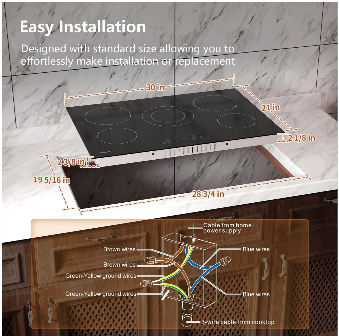
Image: A detailed diagram illustrating the cooktop's overall dimensions (30 inches wide, 21 inches deep, 2 3/8 inches high) and the precise cut-out dimensions required for installation (28 3/4 inches wide, 19 5/16 inches deep). A wiring diagram for a 3-wire cable from the cooktop to the home power supply is also shown.
