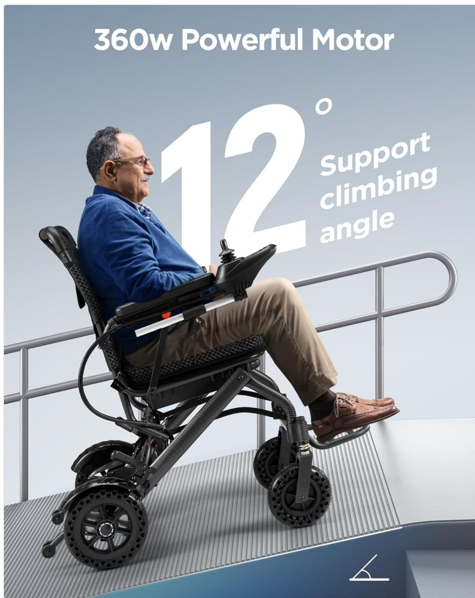
Figure 3.2: The wheelchair demonstrating its climbing capability on a 12-degree incline.
