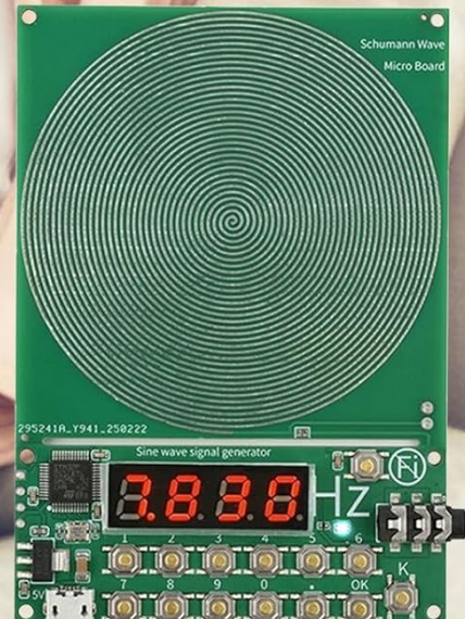
Figure 5: The device can output Schumann wave signals via an audio connection, allowing frequencies to be perceived through headphones.
