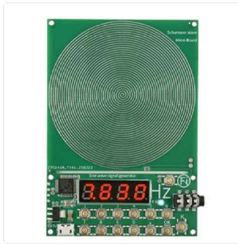
Figure 3: Close-up view of the digital display and spiral antenna on the circuit board.
