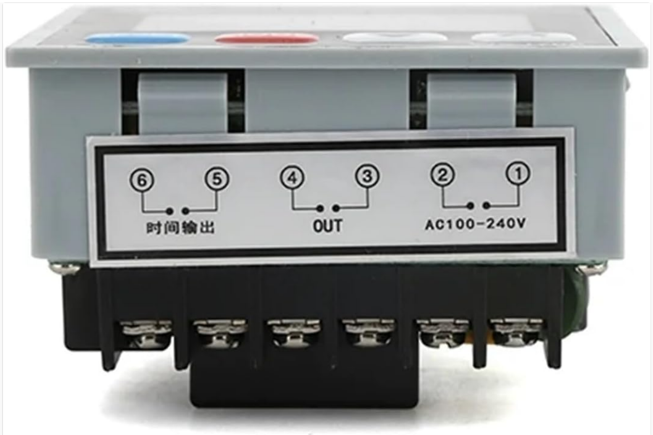
Figure 5: Rear view of the WSJ700 Temperature Controller, illustrating the external wiring terminals. Labels indicate connections for AC100-240V (terminals 1, 2), OUT (terminals 3, 4), and Time Output (terminals 5, 6).
