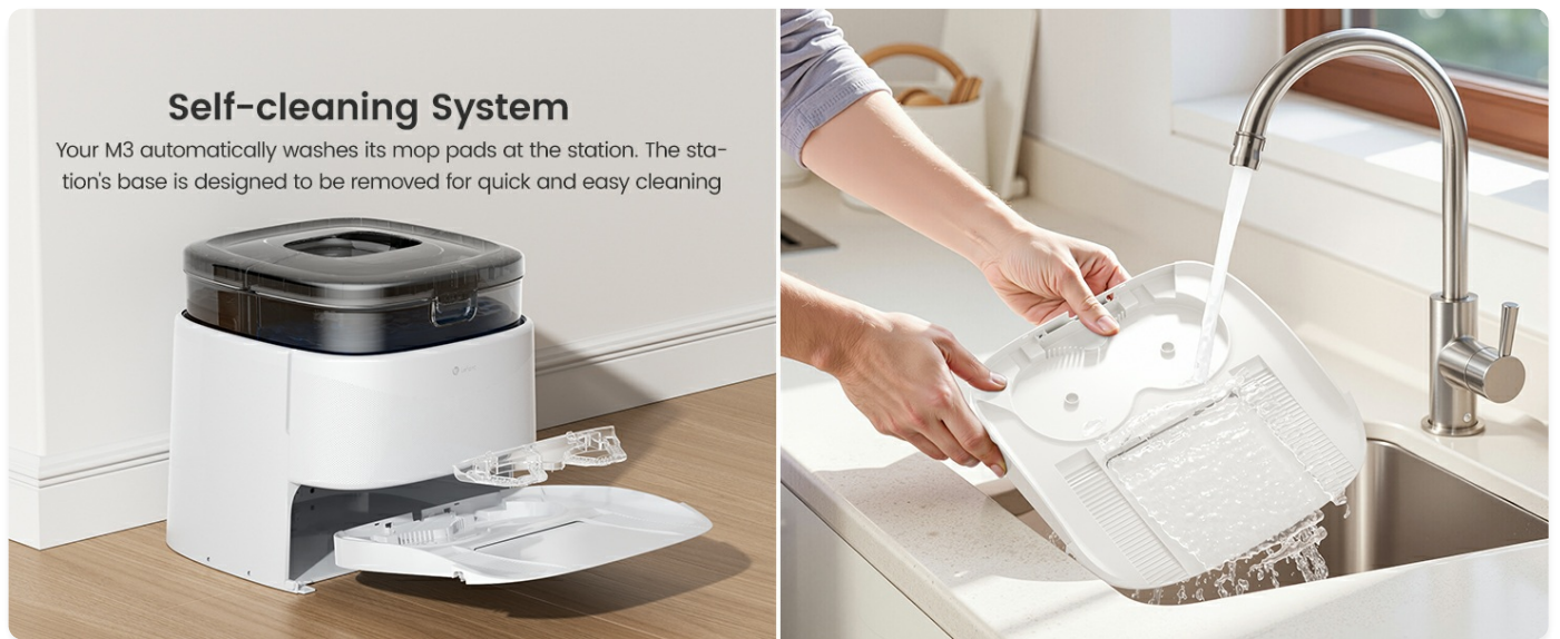
Figure 14: The Lefant M3's self-cleaning system, showing the robot washing its mop pads at the station and the removable base for easy manual cleaning.
