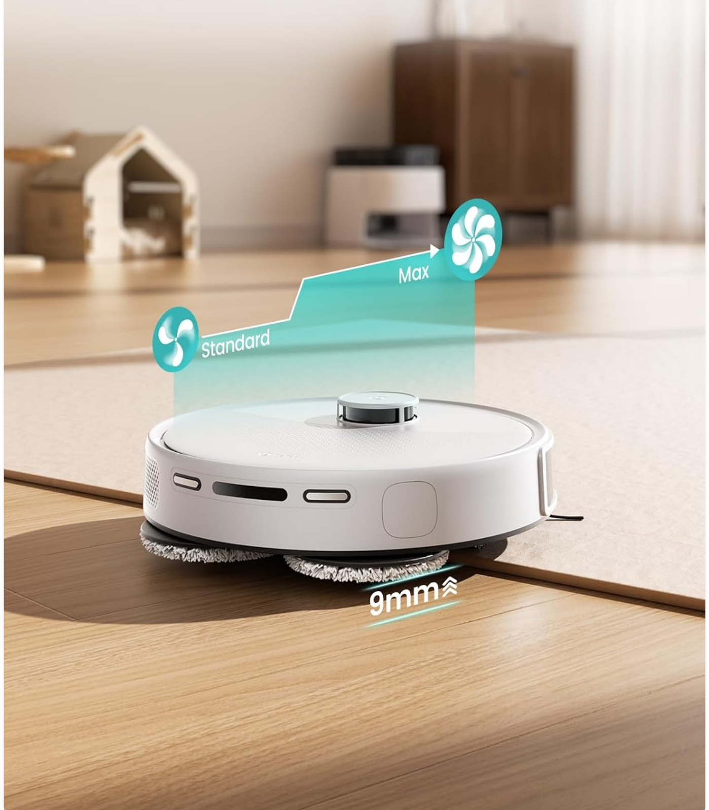
Figure 8: The Lefant M3's auto-lift mopping feature, showing the mop lifting by 9mm when detecting carpets and boosting suction.
