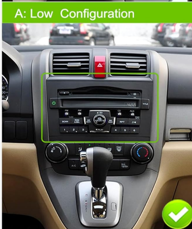
Image 3.2: Comparison of Honda CRV dashboard configurations. Option A (Low Configuration) is compatible, while Option B (High Configuration) is not.
