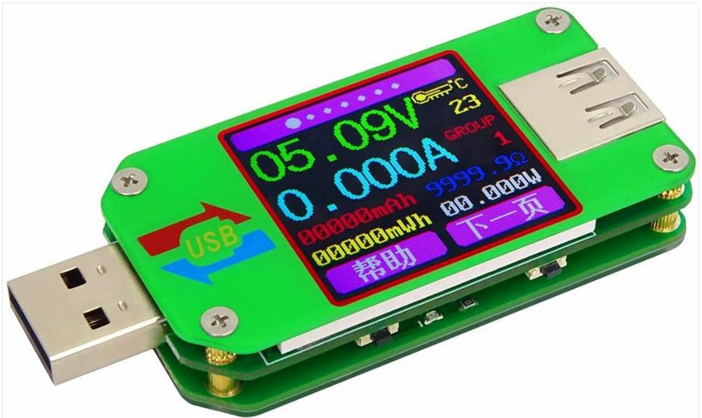
Figure 1: Front view of the Ruideng UM24C USB Tester, displaying real-time voltage (05.09V) and current (0.000A) measurements, along with temperature and accumulated capacity (mAh, mWh) on its color screen. The USB input and output ports are visible.
