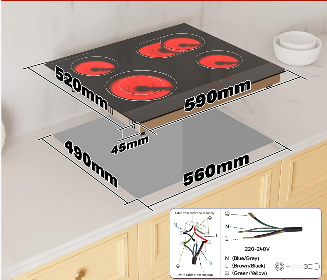
Image: Installation dimensions and electrical wiring diagram.
