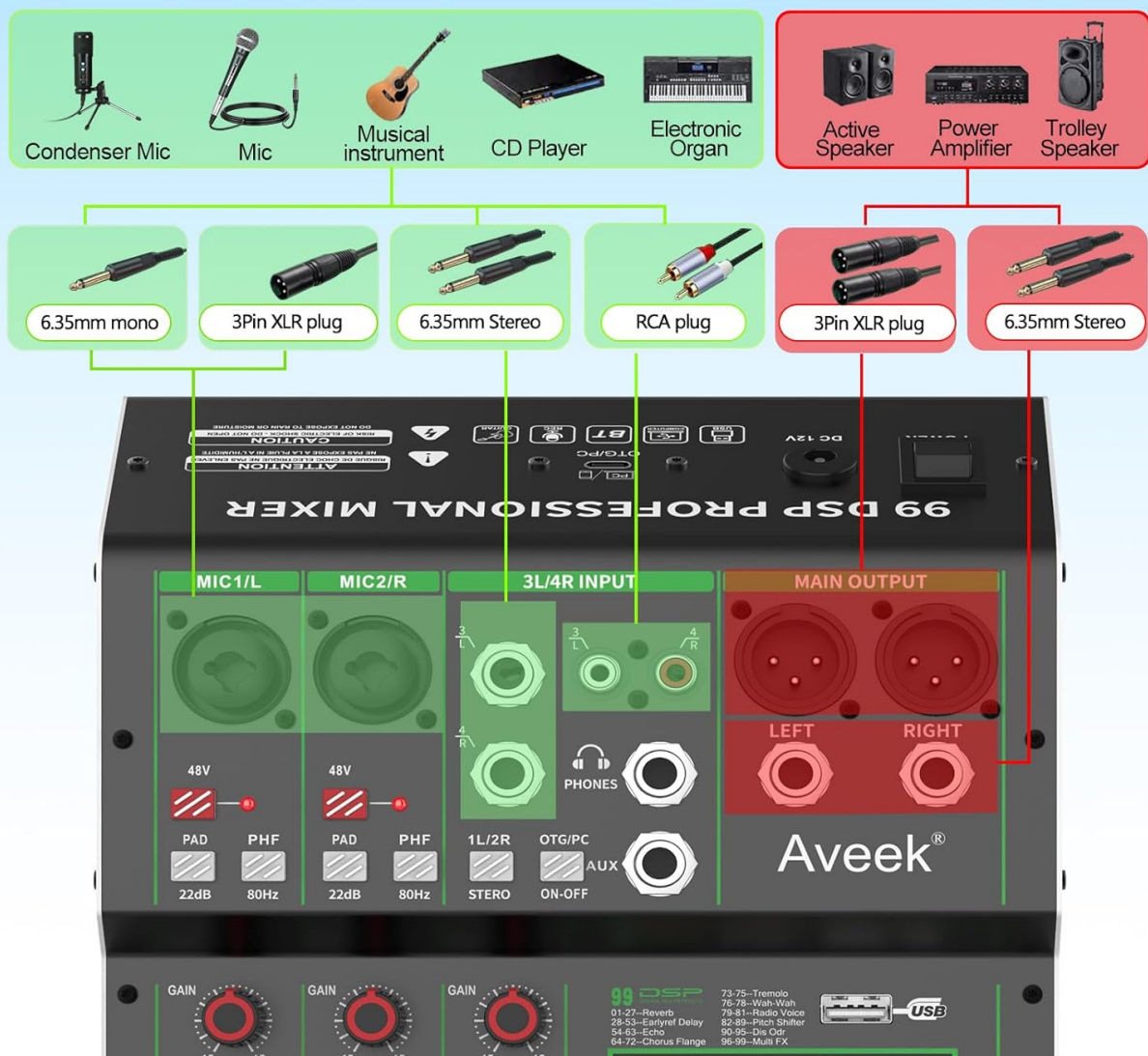
Image: Visual guide showing various compatible input devices (condenser mic, mic, musical instrument, CD player, electronic organ) and their corresponding cable types (6.35mm mono, 3-pin XLR, 6.35mm stereo, RCA plug).
