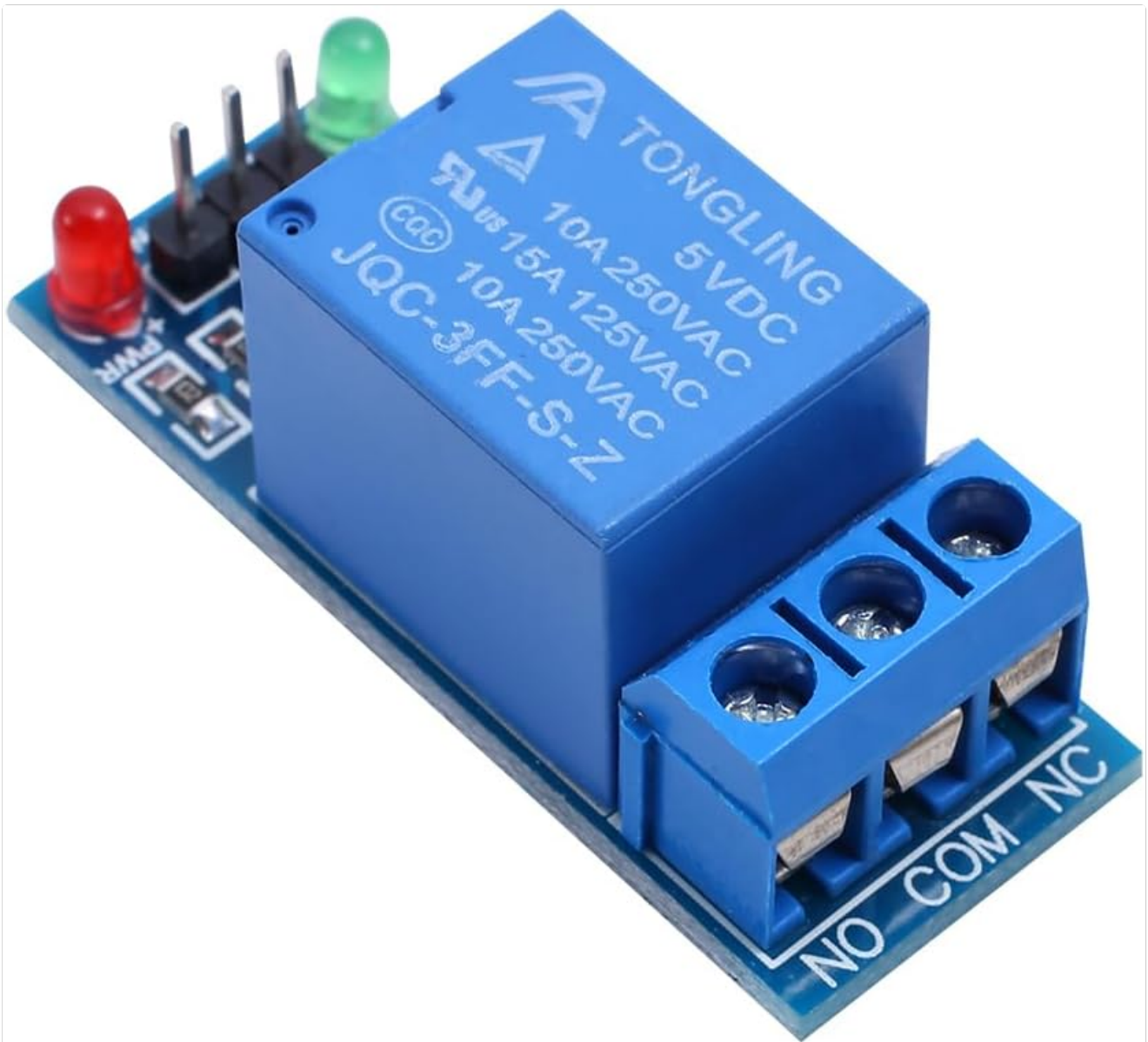
Figure 5.2: Output side of the relay module, showing NO, COM, and NC terminals.
