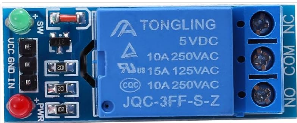
Figure 2.1: Top view of the Teyleten Robot 1 Channel Relay Module, showing the relay, input pins, and output terminals.
