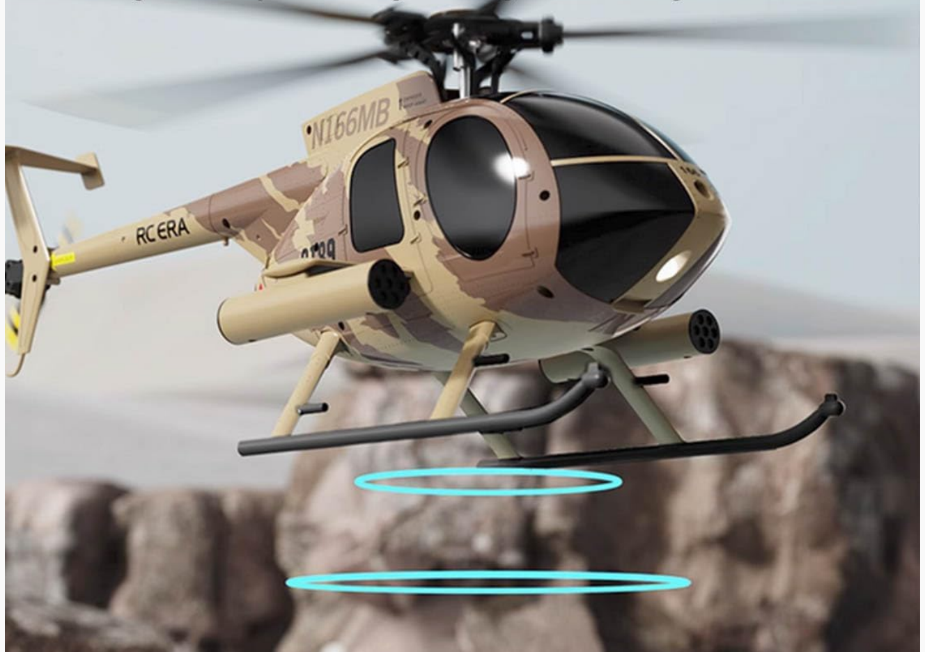
Image 5.2: The helicopter demonstrating stable hovering due to its air pressure fixed altitude flight system.
