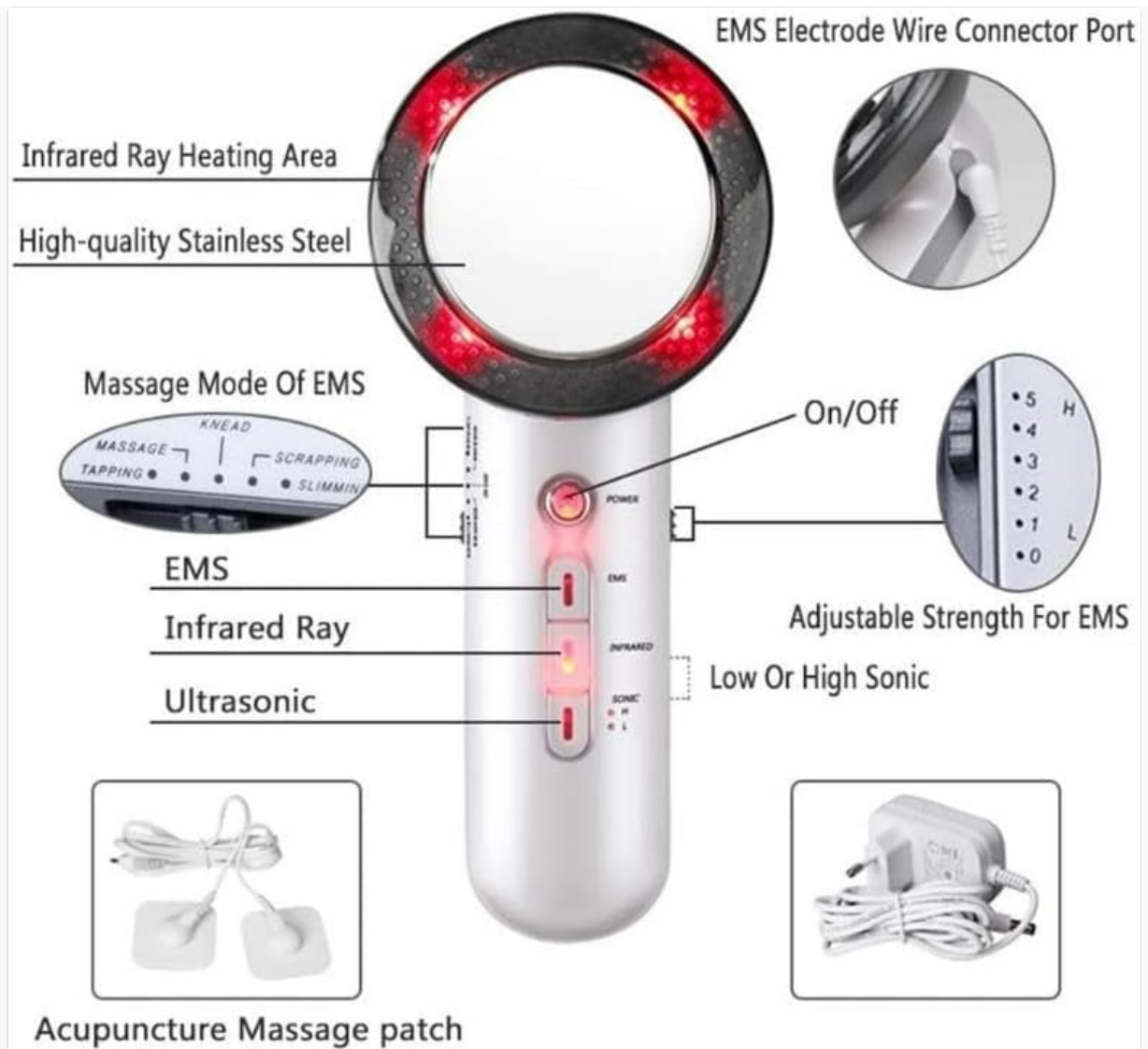
Image: Detailed diagram illustrating the various components and controls of the device, including the On/Off button, EMS, Infrared, and Ultrasonic indicators, EMS mode selector, adjustable strength dial, infrared ray heating area, and the EMS electrode wire connector port.
