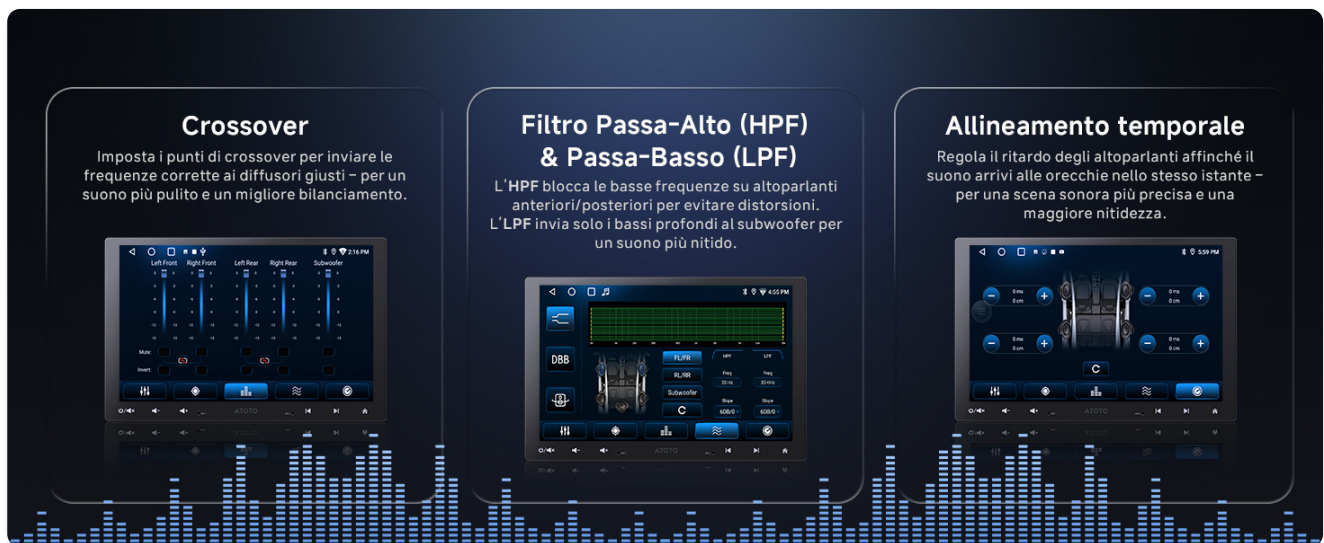
Figure 6: DSP settings interface for Crossover, HPF/LPF, and Time Alignment.
