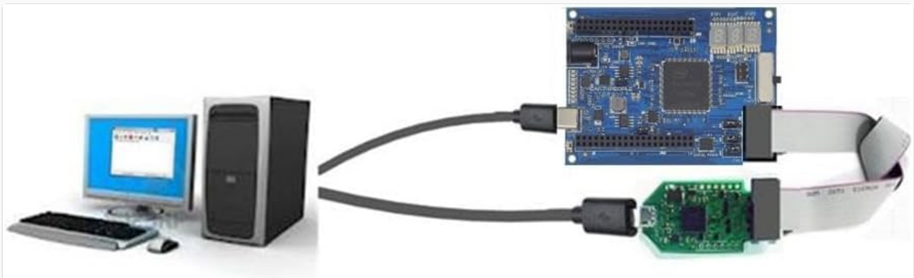
Figure 2.2: Typical setup showing the CycloFlex board connected to a computer and a JTAG programmer for development.
