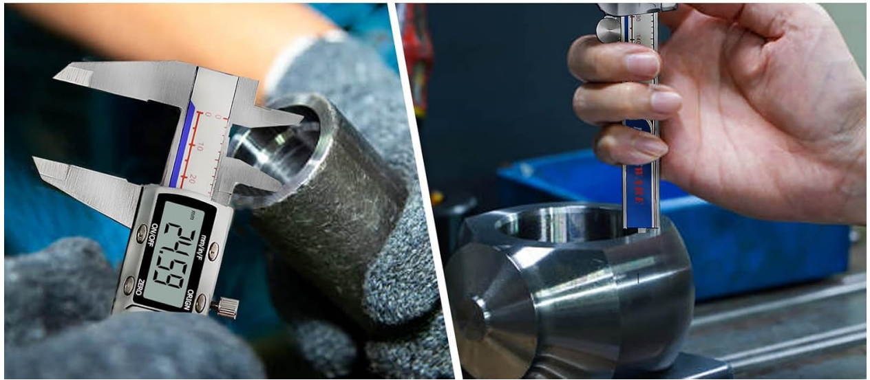
Figure 5: Composite image illustrating external, internal, step, and depth measurement methods.
