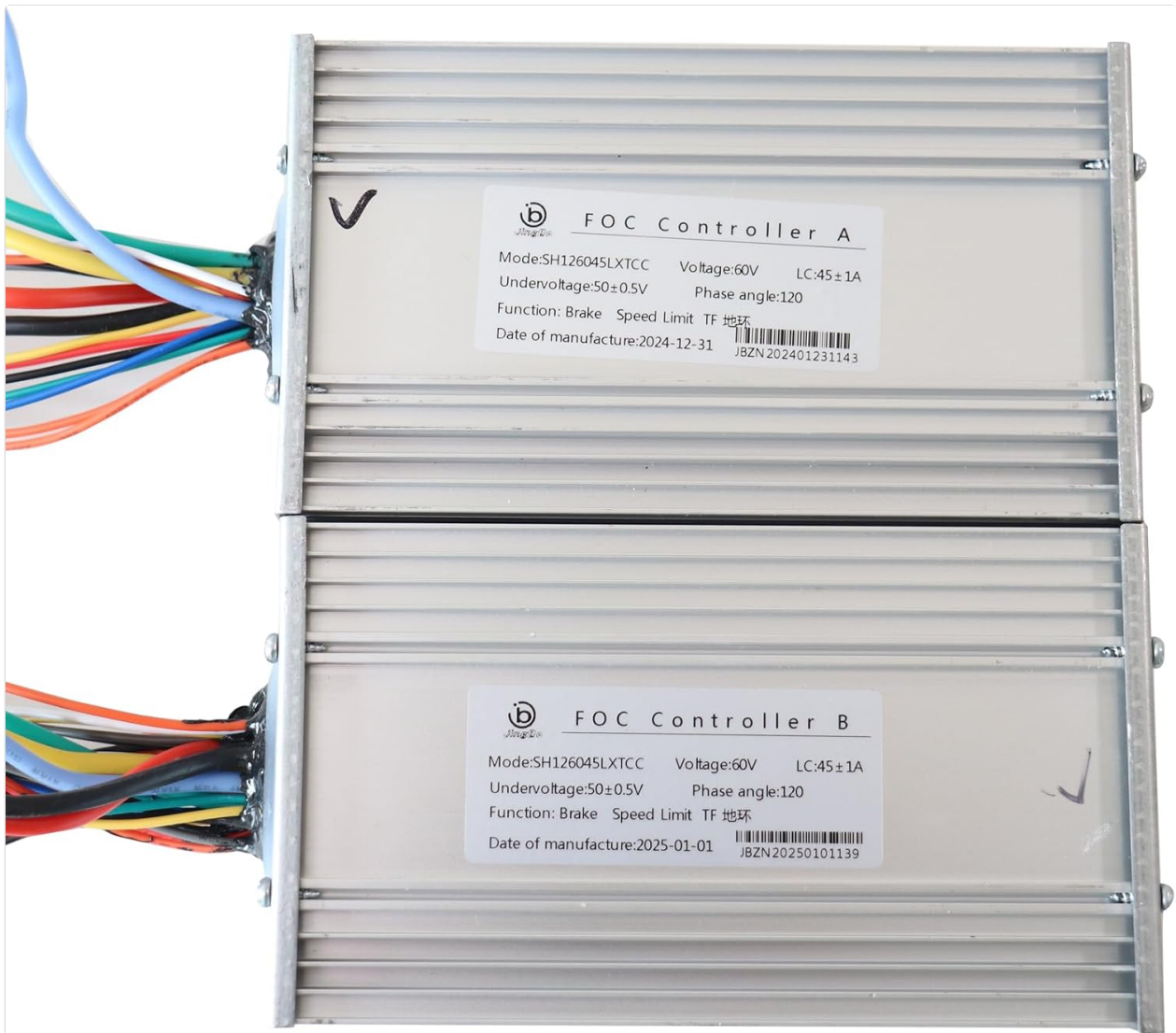
Image: Close-up view of the labels on FOC Controller A and FOC Controller B, showing model numbers, voltage, undervoltage, and manufacturing dates.
