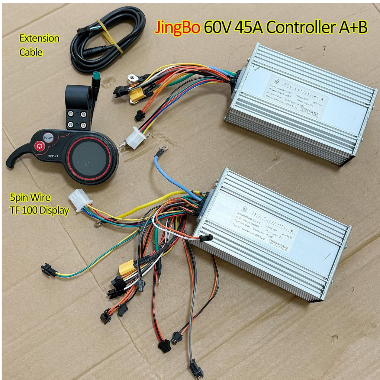
Image: The complete set including both controllers, the TF-100 display, and an extension cable, illustrating how they connect.
