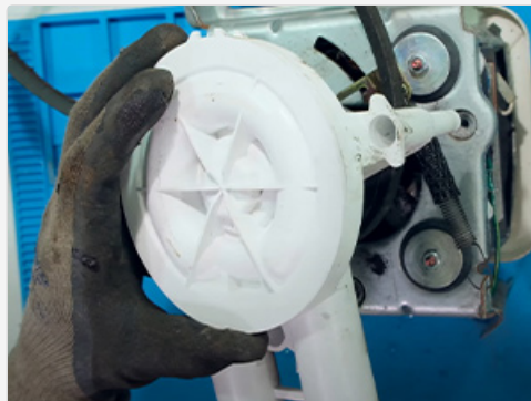
Image 4.2: Step 2 - Taking off the water pump.
