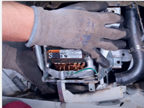
Image 4.1: Step 1 - Removing the washing machine motor.
