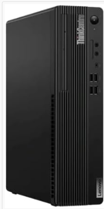
Figure 3.2.2: Front view of the desktop, showing the accessible USB-C, USB-A, and headphone/mic combo ports.
