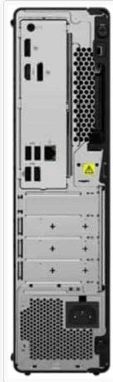
Figure 3.2.1: Rear view of the desktop, highlighting the DisplayPort, HDMI, USB-A, and Ethernet ports for connecting peripherals.
