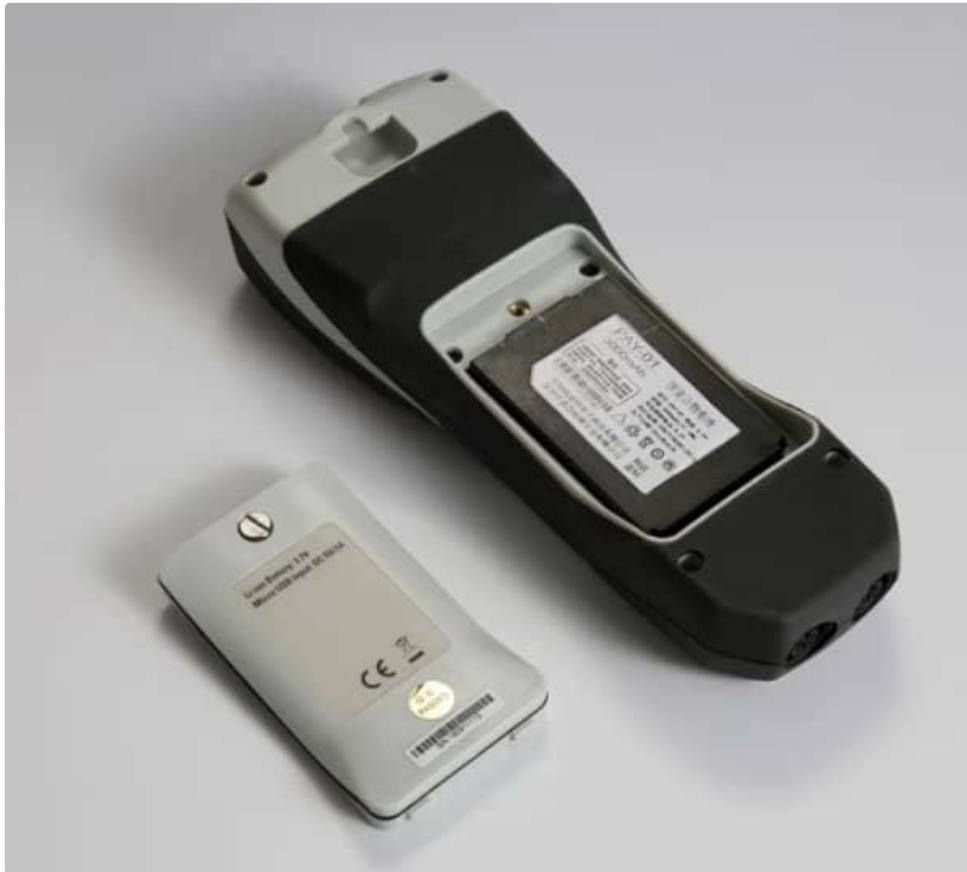
Figure 3: The DT-8321 with its battery compartment open, showing the rechargeable lithium battery.
