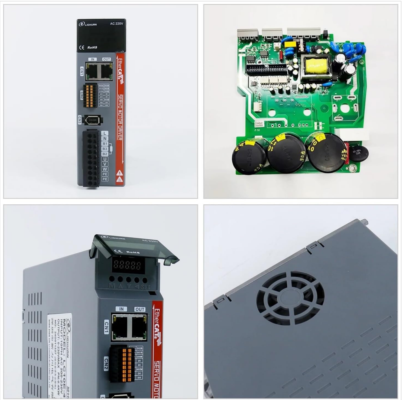
Figure 8.1: Various views of the Lichuan LC10E EtherCAT Servo Motor Driver, showing its front panel, internal circuitry, top view, and cooling fan. These images provide a closer look at the physical design.
