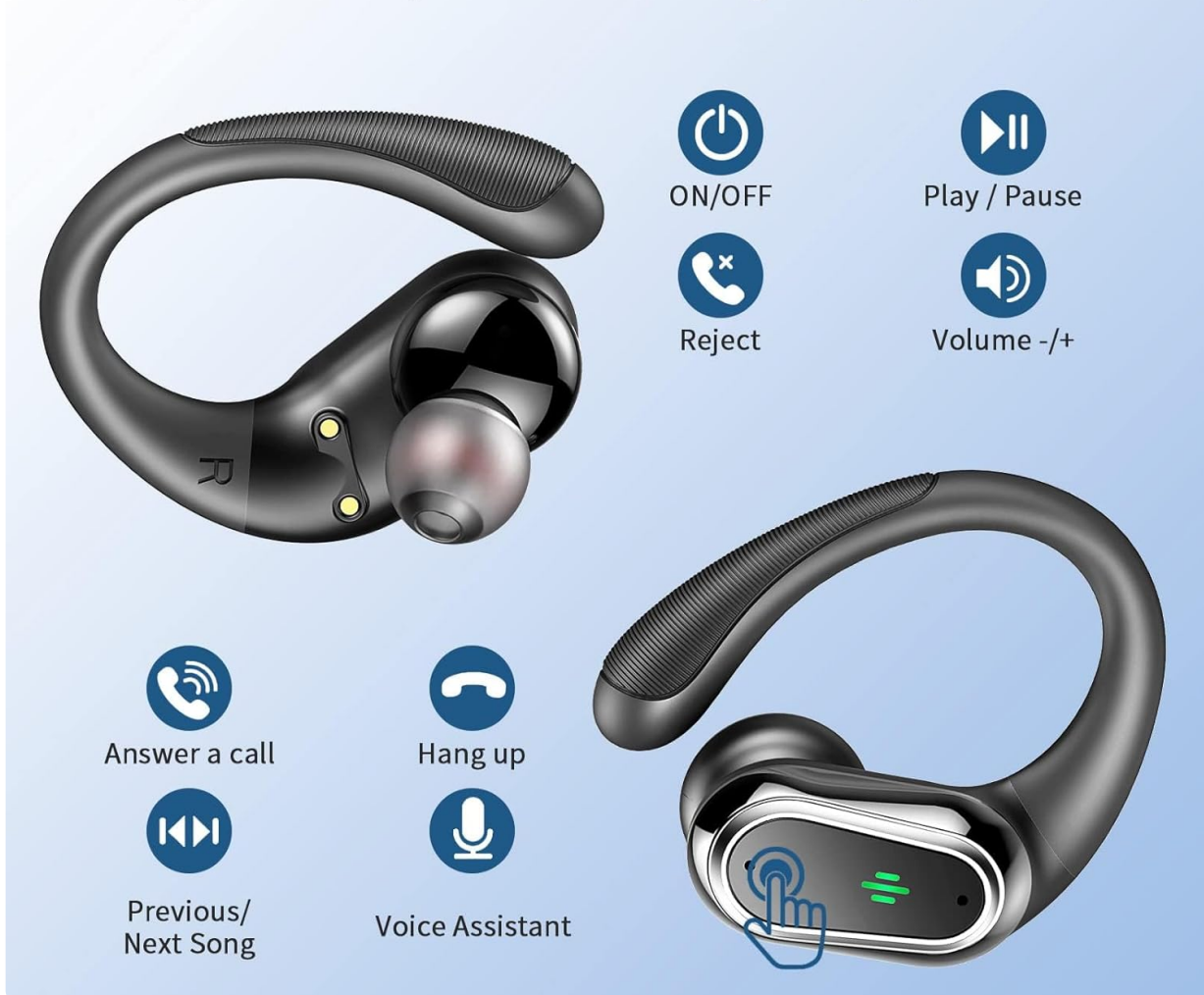
Image 5.1: Diagram illustrating the various smart touch control functions on the earbuds, including power, play/pause, call management, volume, and track navigation.
