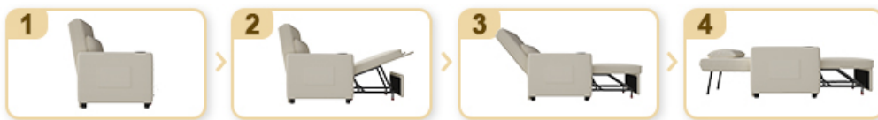
Image: A four-panel diagram illustrating the mechanism for converting the sofa into a bed, showing the pull-out and unfolding steps.
