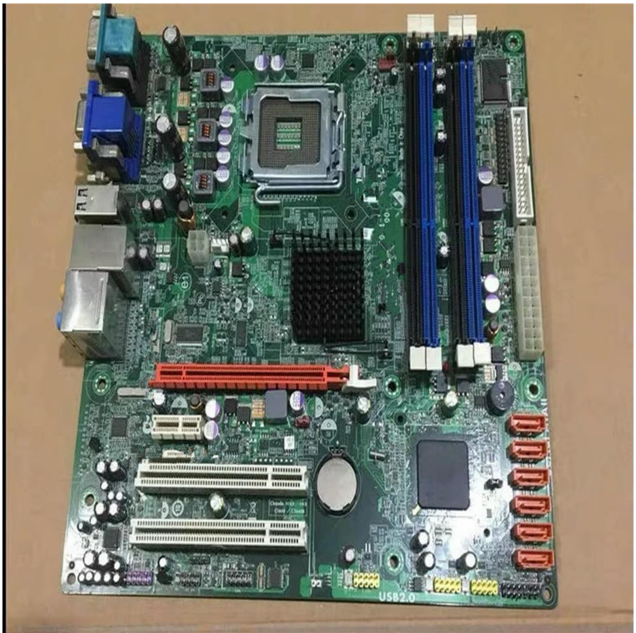
Figure 3.1: Generic Q45T-CM Main Board Layout. This image displays the motherboard from a top-down perspective, highlighting key components such as the LGA 775 CPU socket at the top-center, two blue and two black DDR3 RAM slots to its right, and various expansion slots (PCIe x16, PCI) towards the bottom. The rear I/O panel with DVI, VGA, and USB ports is visible on the left edge, while multiple orange SATA ports are arranged along the right edge. The main 24-pin ATX power connector is located on the upper right, and the 4-pin CPU power connector is near the top left.
