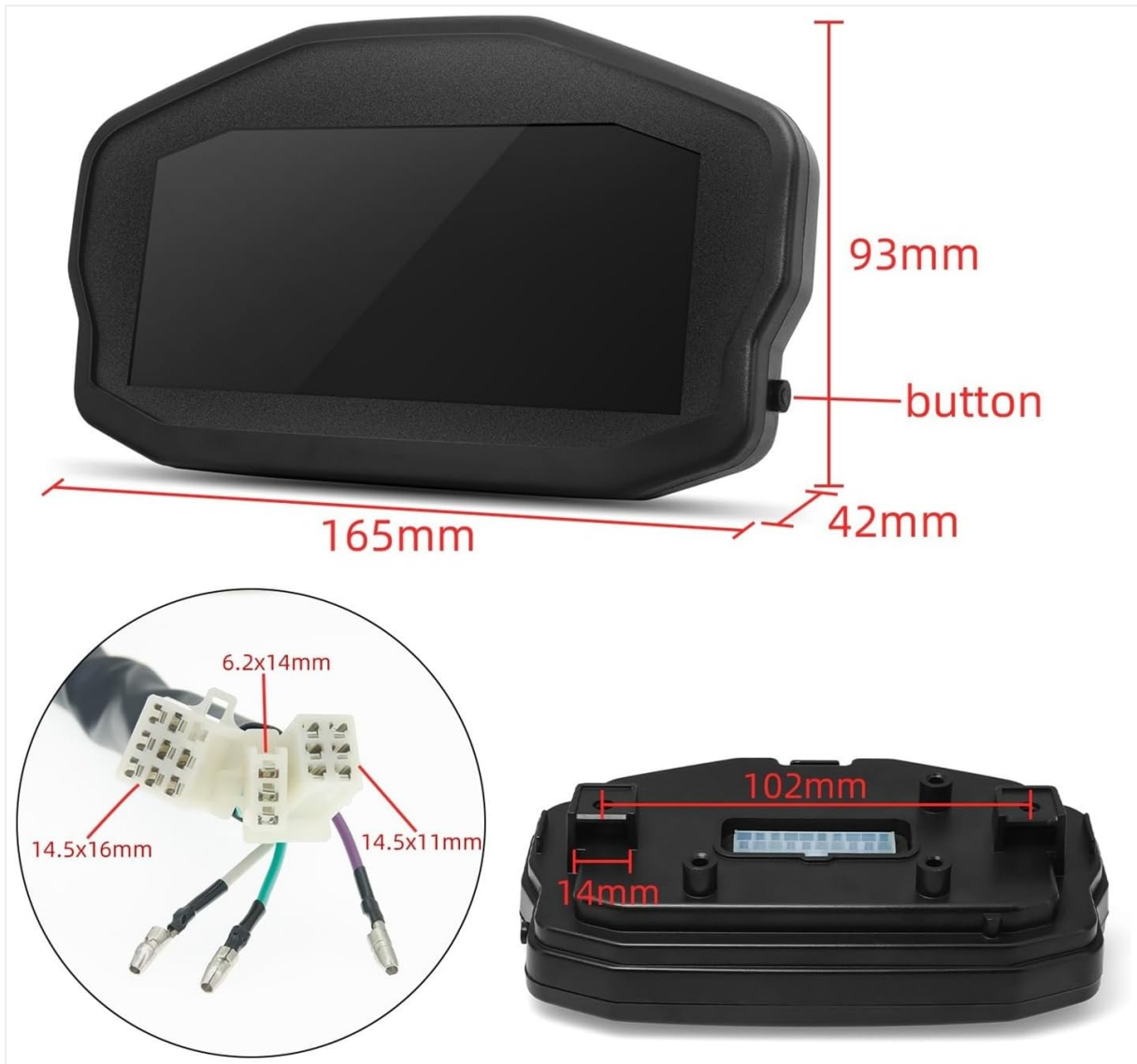
Figure 4: Product dimensions and wiring harness details. Refer to this diagram for correct wire identification and connection points.
