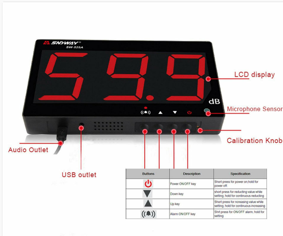
Figure 1: SW-525A Sound Level Meter with labeled parts and control buttons.
