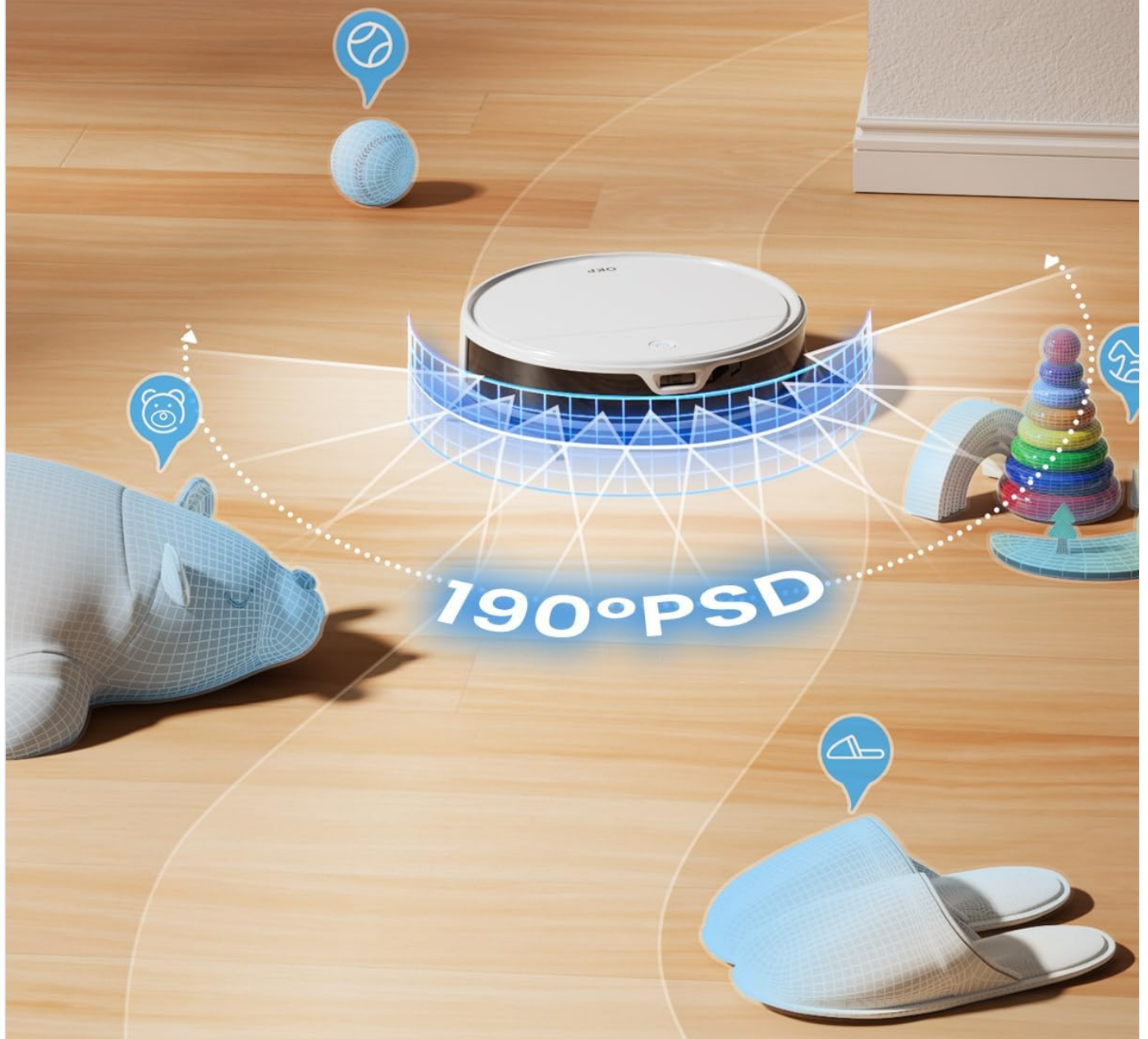
Figure 5: Precise PSD sensors enable the robot to avoid obstacles and prevent collisions.
