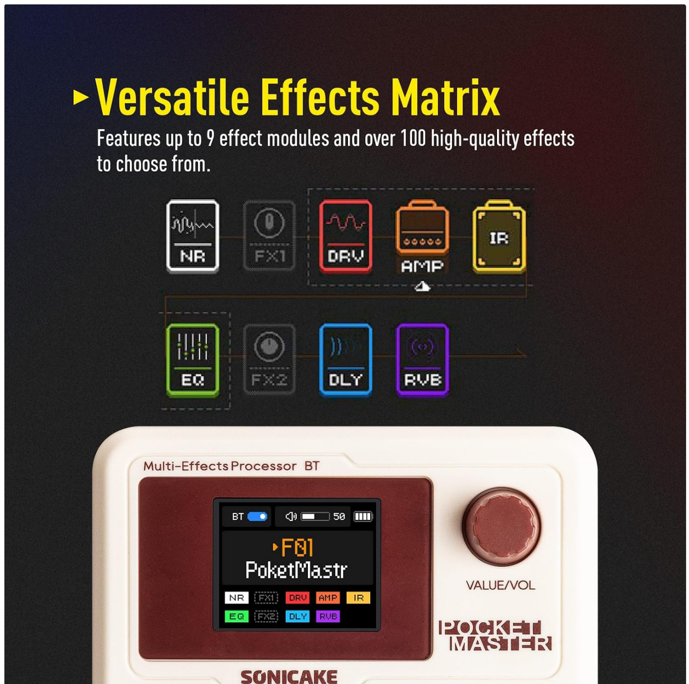
Image: The Pocket Master's display illustrating the versatile effects matrix with various effect blocks.
