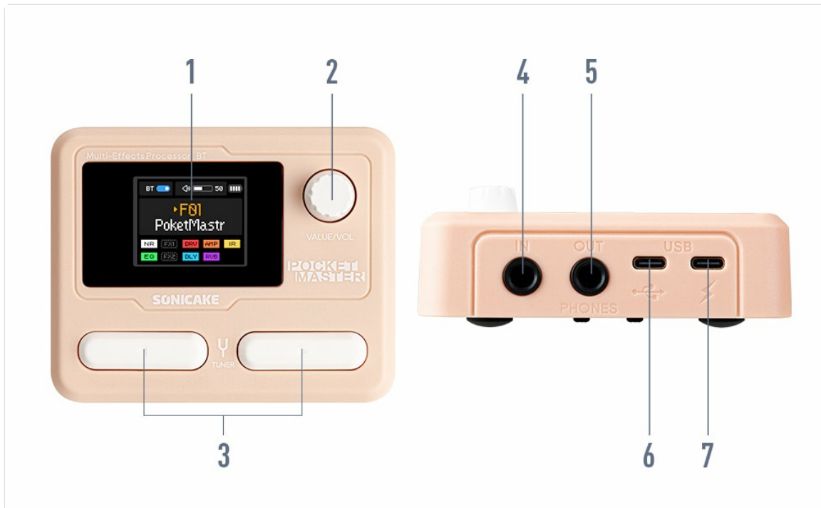
Figure 2.2.2: Side view of the SONICAKE Pocket Master, illustrating the input (IN), output (OUT), headphones (PHONES), and USB ports (USB-C for data/power, USB-A for OTG).
