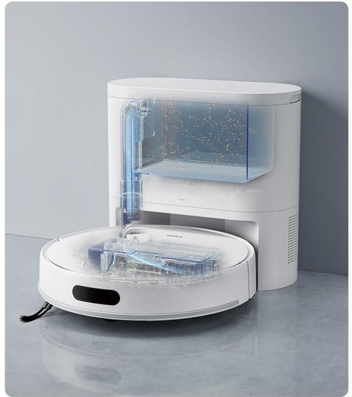
Figure 3.4: This image illustrates the automatic dust collection system, featuring a large 4-liter dust bag being inserted into the charging dock.
