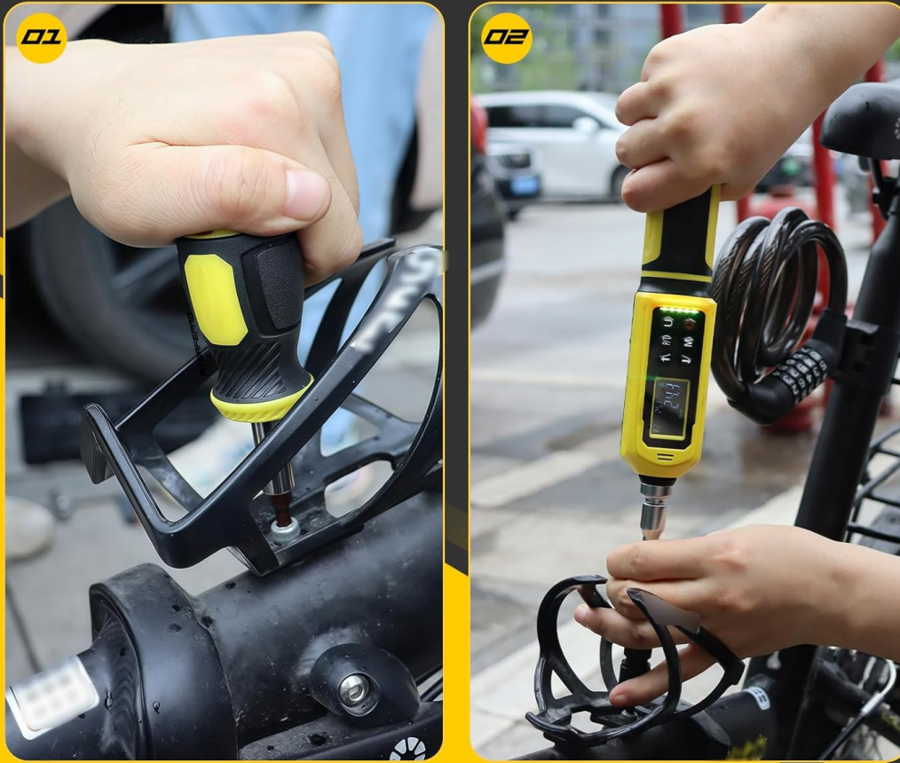
Image 4.1: The image illustrates the two-step process: using the standard handle for initial quick fastening (left) and the digital torque screwdriver for final precise tightening (right).
