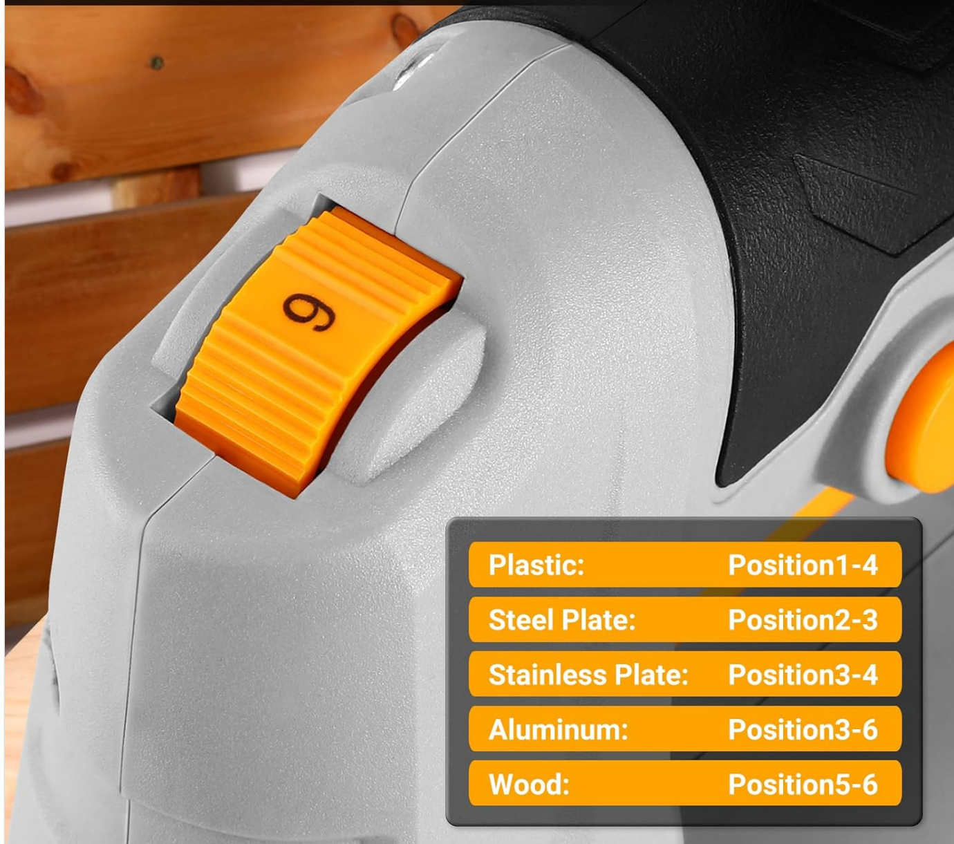
Image 5.2: The 6-speed dial with recommended settings for various materials, ensuring optimal cutting performance.
