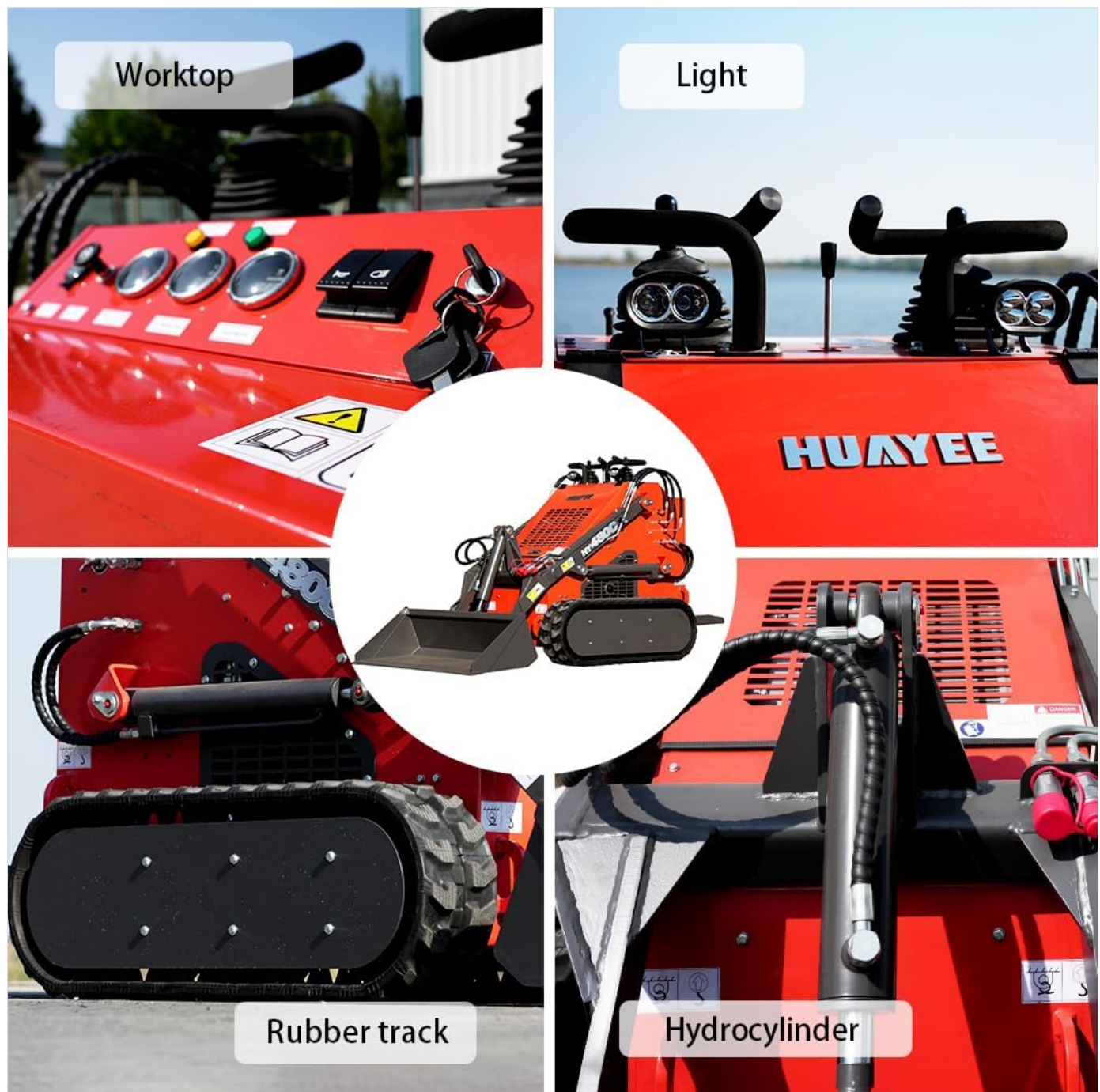
Figure 3.4: Close-up images illustrating the control worktop, front work lights, durable rubber track, and the hydraulic cylinder (hydrocylinder).
