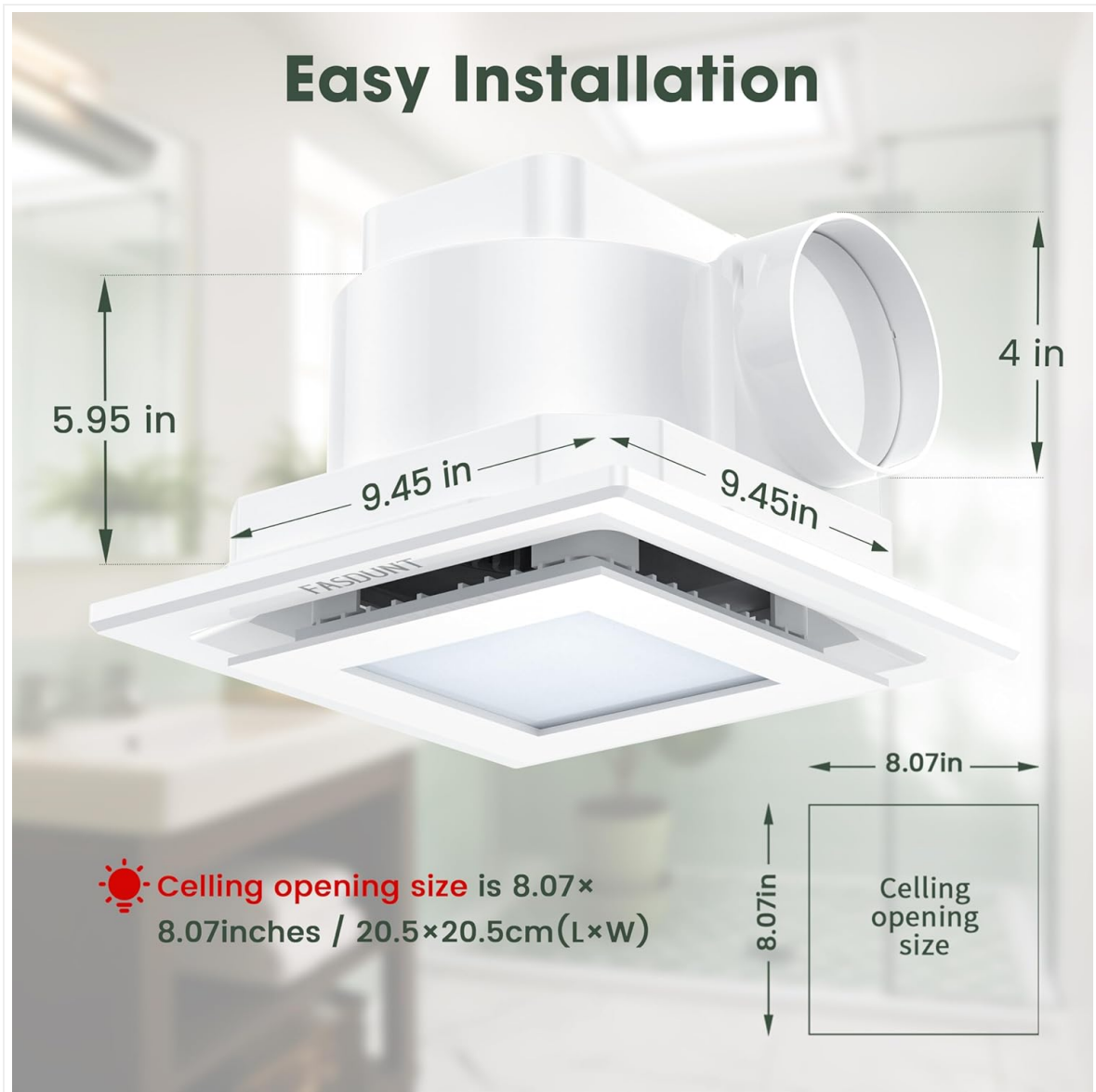
Image 4: Diagram showing fan dimensions and required ceiling opening size.
