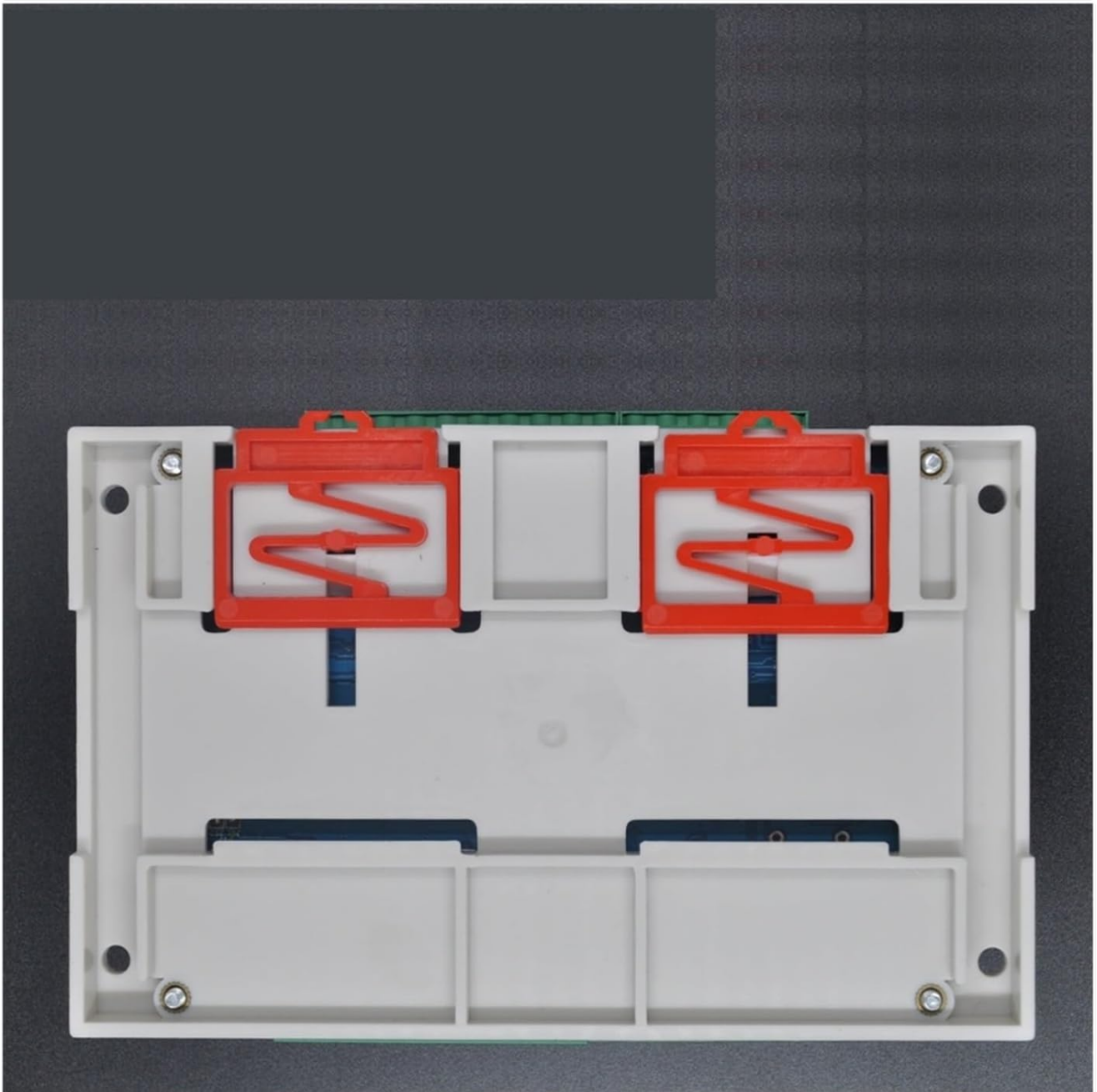
Figure 4.1: Rear view of the module, illustrating the integrated clips for 35mm DIN-rail mounting.
