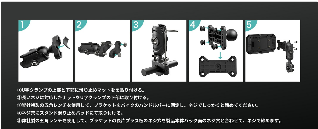
Image: Diagram illustrating the steps for handlebar mounting.
