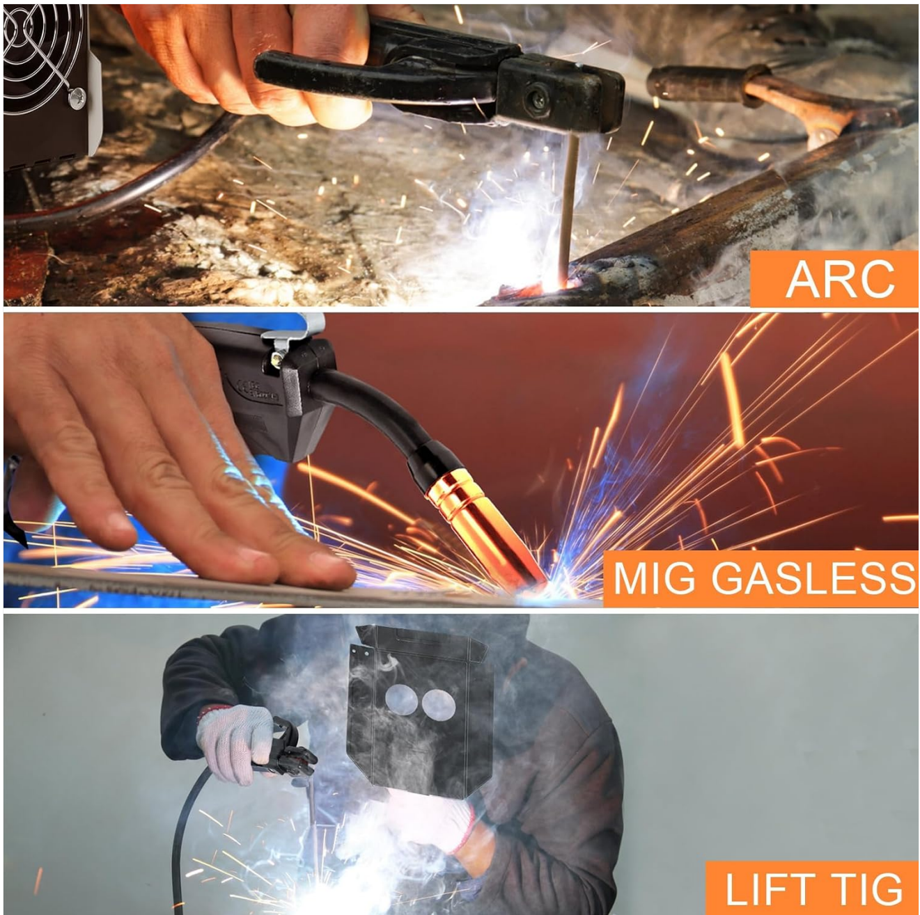
Figure 7.1: Visual representation of the three welding processes supported by the MIG-270: ARC (MMA/Stick) welding, MIG Gasless welding, and Lift TIG welding.
