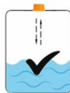
Image: Step-by-step diagrams illustrating the correct and incorrect methods for installing the sensor, emphasizing perpendicular alignment and avoiding obstacles or water inlets.
