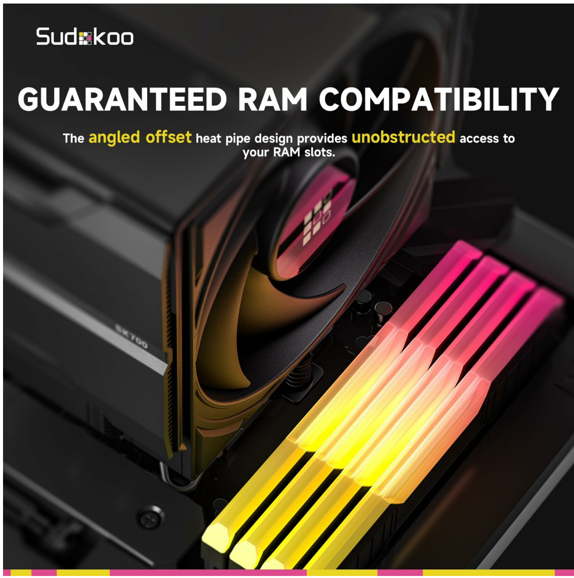
Figure 5.4: Full RAM Clearance with SK700 Cooler
