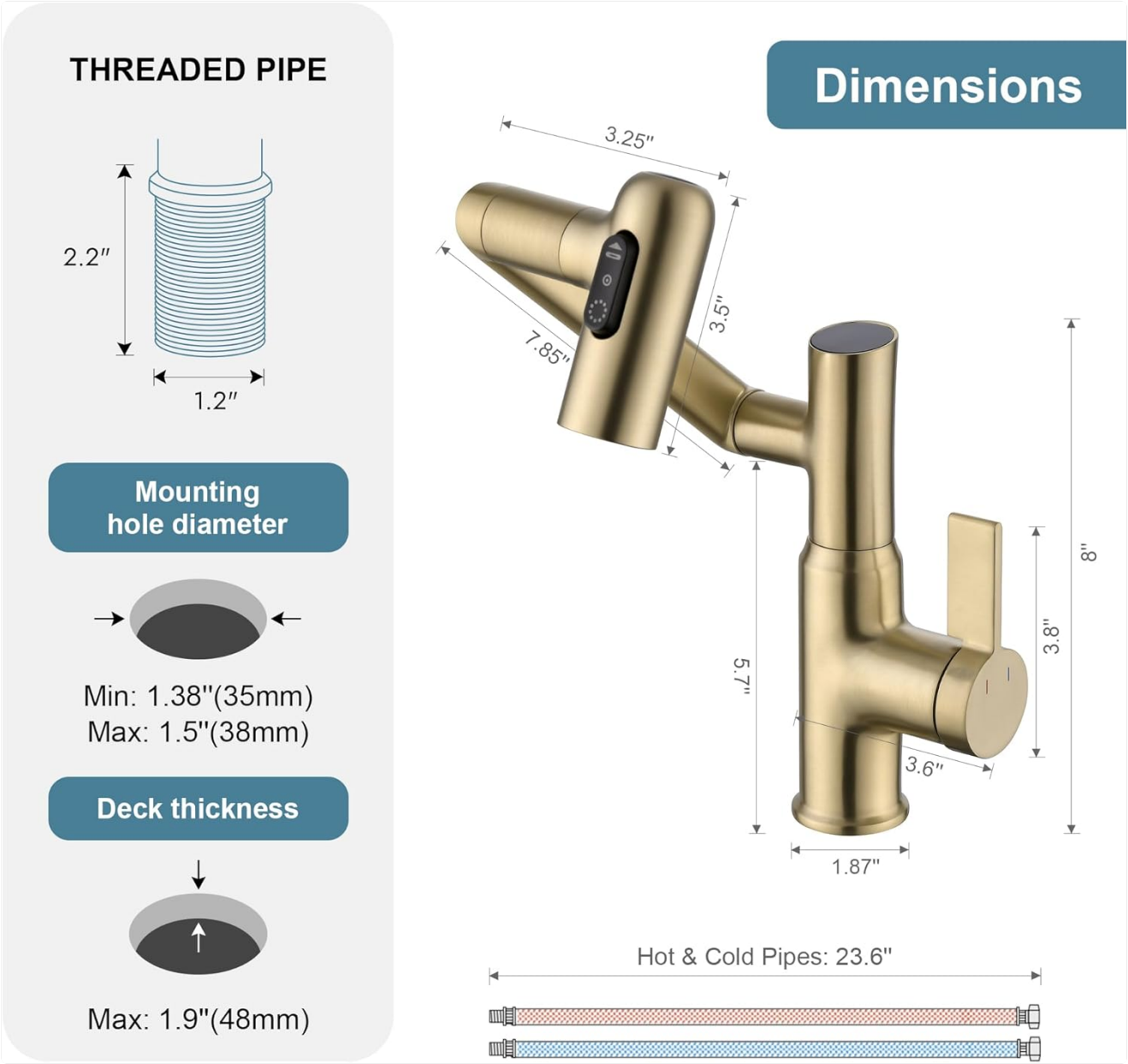
Image 3.1: Detailed dimensions of the faucet, including spout reach, height, and base measurements. Note the mounting hole diameter requirements (Min: 1.38"/35mm, Max: 1.5"/38mm) and maximum deck thickness (1.9"/48mm).
