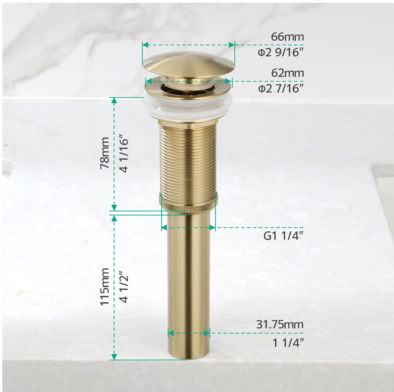
Image 3.2: Detailed dimensions of the pop-up stopper, showing its overall height, cap diameter, and thread size (G1 1/4").
