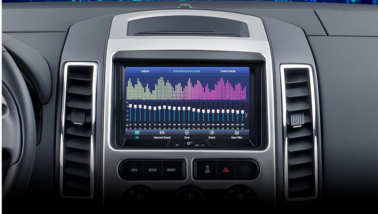
Figure 5.4: Intelligent Tone Adjustment System. This image displays the DSP settings screen, allowing users to customize sound characteristics.
