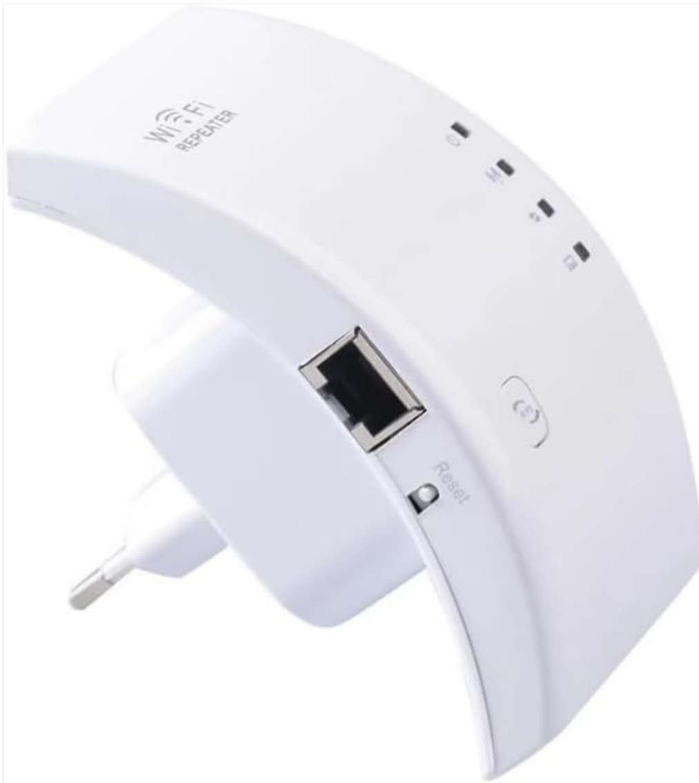
Image 2.2.2: Side view of the WiFi Repeater highlighting the Ethernet port and the recessed Reset button.
