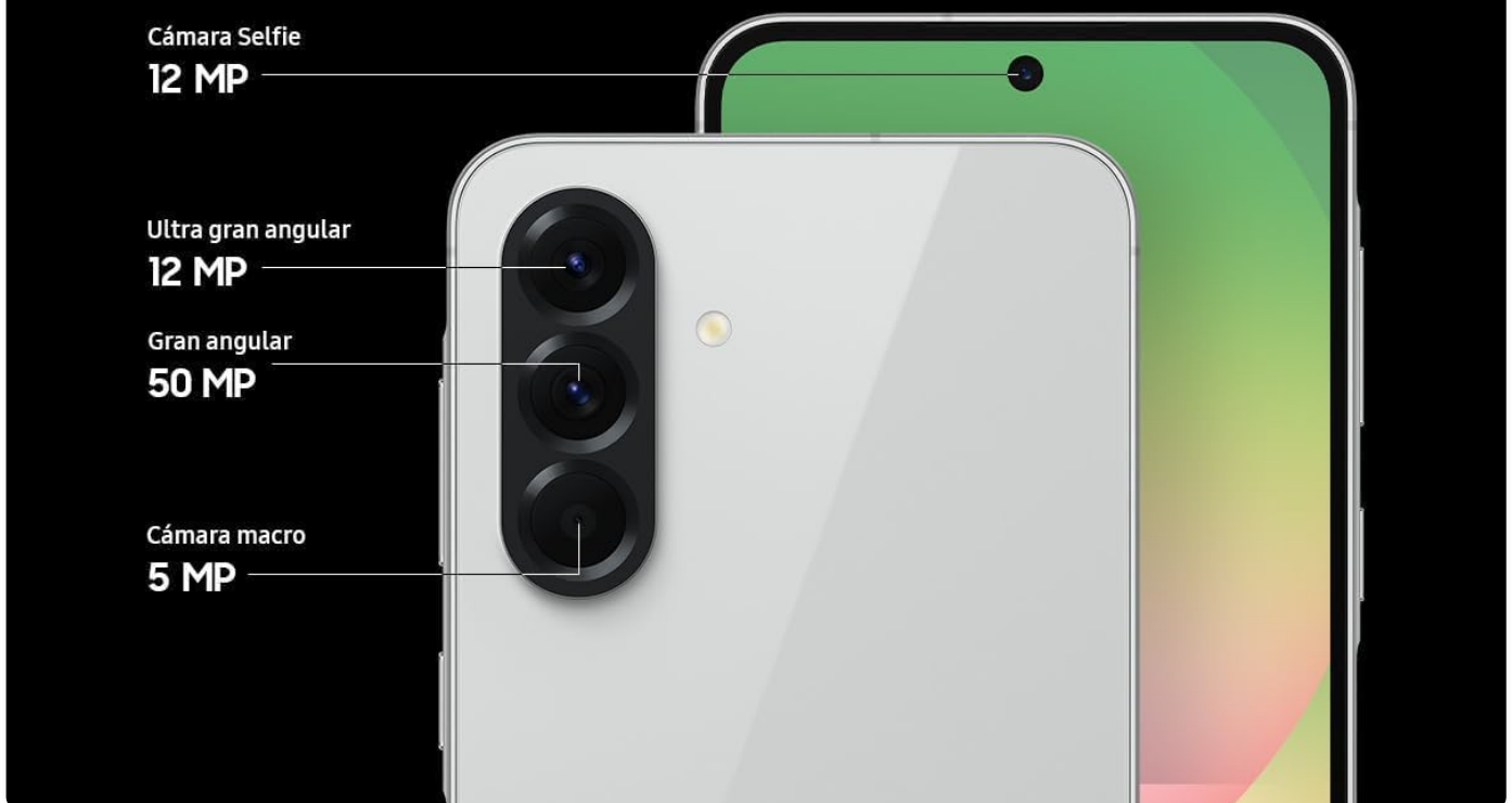
Figure 2: Detailed view of the Galaxy A56 5G camera system, highlighting the 50MP main, 12MP ultra-wide, 5MP macro, and 12MP selfie cameras.
