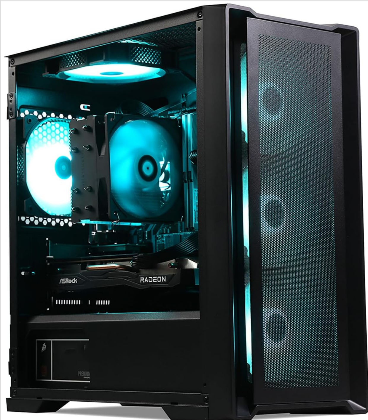
Image 2.1: MXZ Gaming PC with its side panel open, revealing the internal components illuminated by blue RGB lighting. The CPU cooler, RAM, and graphics card are clearly visible.
