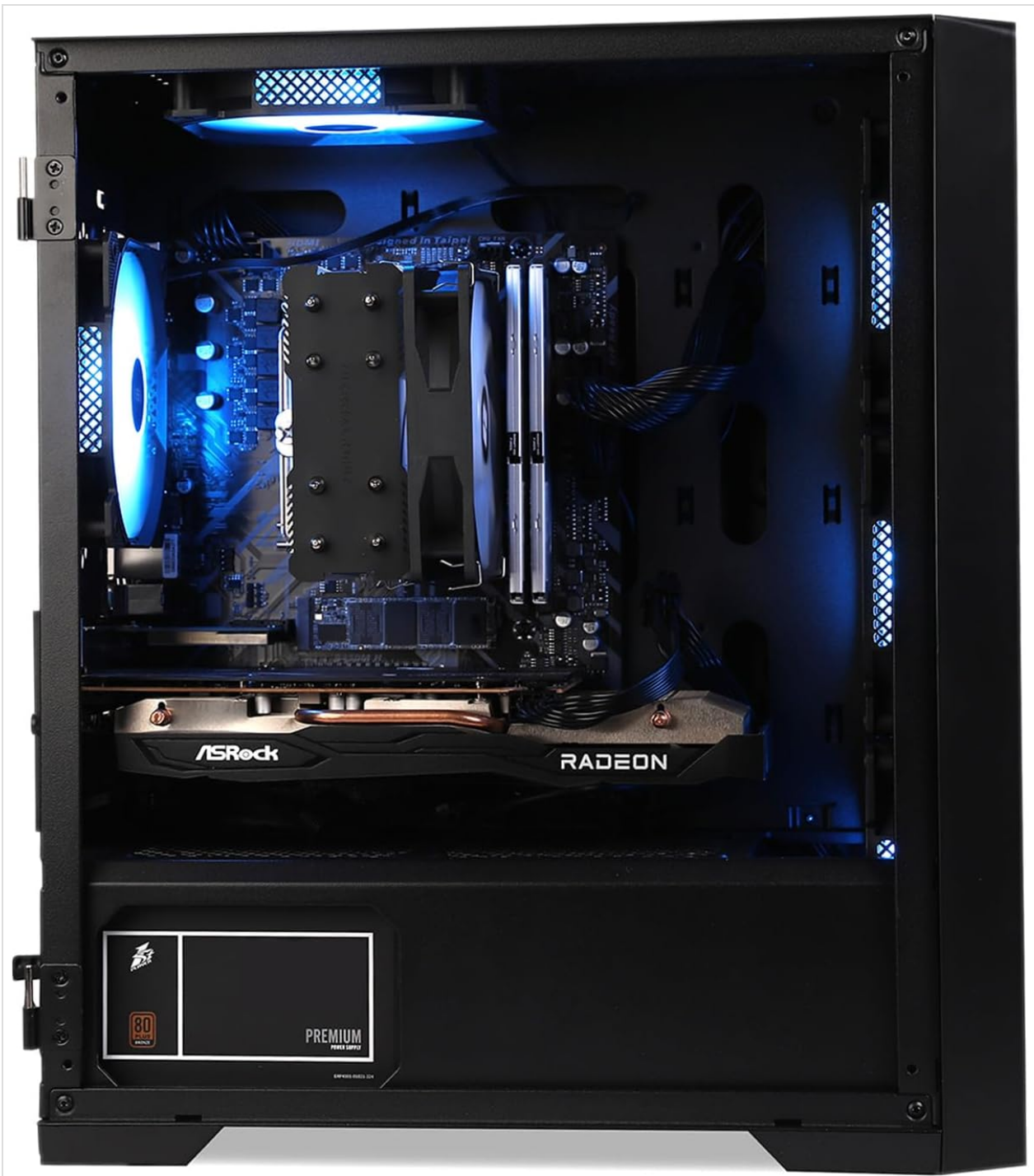
Image 7.1: An internal view of the MXZ Gaming PC, showcasing the arrangement of key components such as the motherboard, CPU cooler, RAM modules, and the dedicated graphics card.
