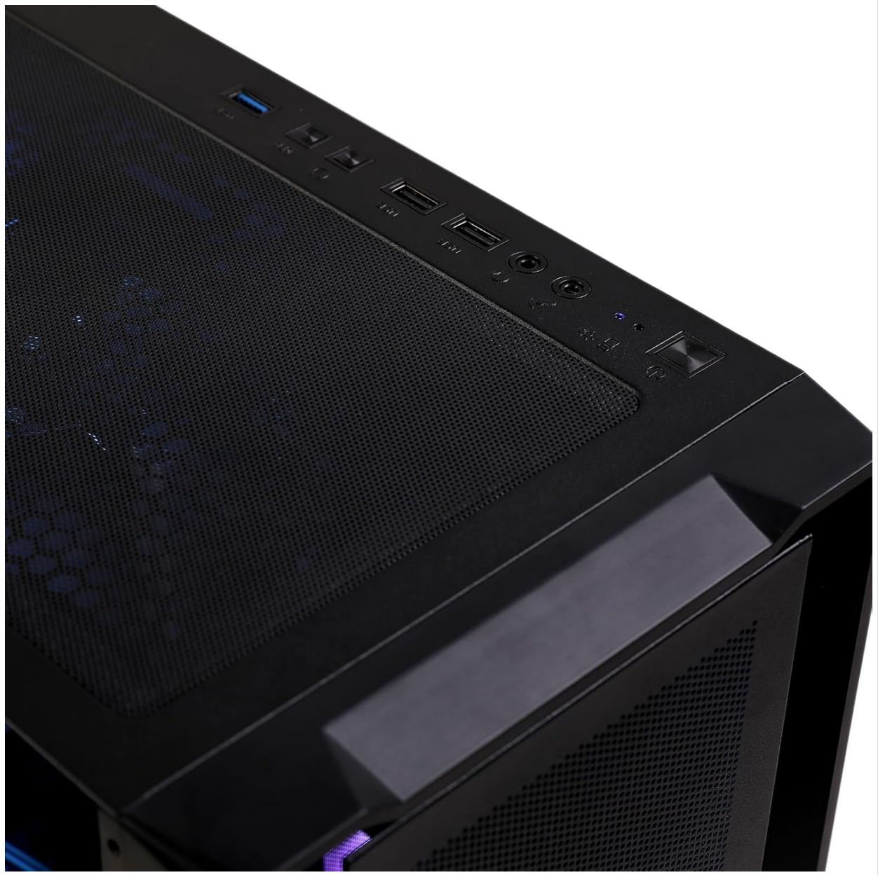
Image 4.1: A close-up of the top front panel of the MXZ Gaming PC, highlighting the power button, USB ports, and audio jacks for convenient access.
