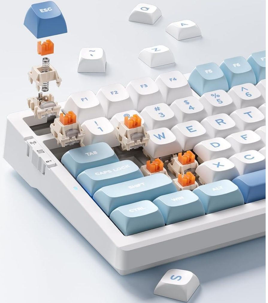
Figure 6: Illustration of hot-swappable switches on the G98 PRO Keyboard, showing switch removal and installation.
